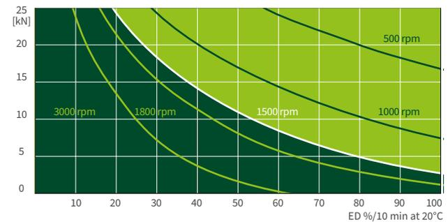
These curves are for guidance under standard industrial conditions (ambient temperature 20°C etc.) and correct maintenance (lubrication etc.). They are based on the ZIMM standard trapezoidal thread Tr 30x6. The operation cycles can be many times longer, when using ball screws.
