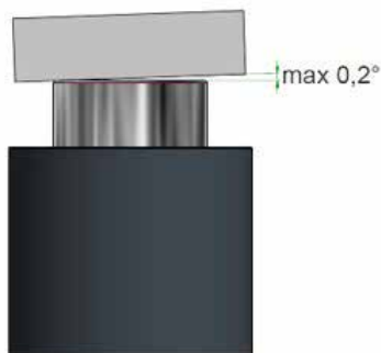
Load is loosely placed
