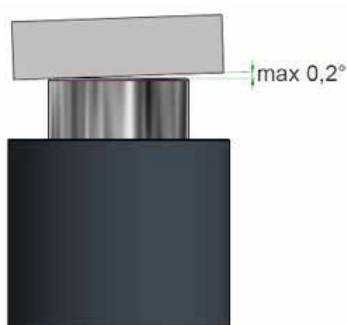
Load is loosely placed
