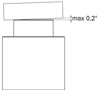
Fig. 1: Load resting loosely
